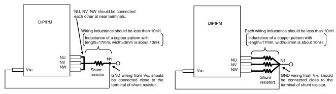
Low inductance shunt resistor like surface mounted (SMD) type is recommended.
