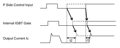
Real line: off pulse width > PWIN(off); turn on time t1 Broken line: off pulse width < PWIN(off); turn on time t2 (t1:Normal switching time)
